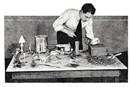
This complete foundry shop for the home workshop will make castings and art objects from practically any metal having a melting point of less than 2,400 degrees F. It uses gas.
