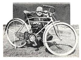
No longer is it difficult to ride a bicycle up hill provided it is equipped with a gear shift like the one shown here. The inventor, William E. Sperry, points out the gear shift control.
