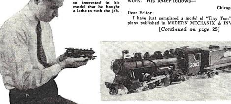
Here is a close-up of Streng's "Tiny Tom." The drive wheels were made up of brass sheets soldered together and turned out on lathe. All parts were made at home except the motor.
