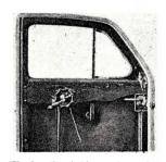
The handle of this car door raises the windows when turned, and opens the door when pulled in.
