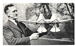
Here is the web-footed airplane which kicks its way through air like a duck through water. The vanes rotate on wheels, and open up on the down-stroke and close on the up-stroke.
