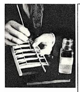
Gluing in the angle braces used to strengthen wing ribs at points of attachment for the bracing wires. Leading edge has been sanded and wing is ready for covering.
